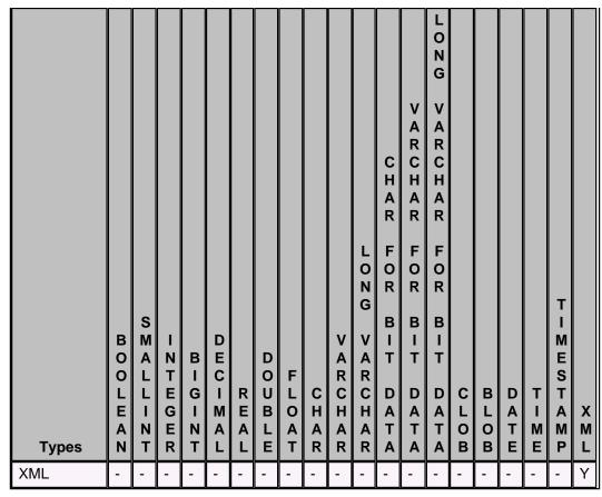
If a conversion is valid, CASTs are allowed. Size incompatibilities between the source and target types might cause runtime errors.
